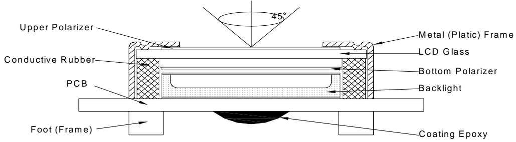
2. View Angle: with in 45° around perpendicular line.
