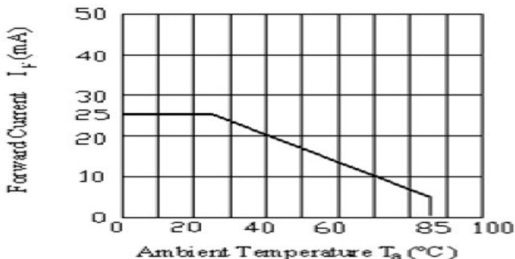
For operation above 25 °C, The  $I_{fm}$  &  $P_d$  must be derated, the current derating is  $-0.36\text{mA}/^\circ\text{C}$  for DC drive and  $-0.86\text{mA}/^\circ\text{C}$  for Pulse drive, the Power dissipation is  $-0.75\text{mW}/^\circ\text{C}$ . The product working current must not more than the 60% of the  $I_{fm}$  or  $I_{fp}$  according to the working temperature.
